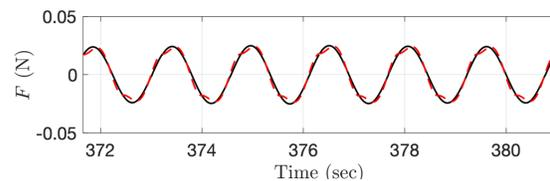
Figure 2 - A comparison of predicted force (red dashed line) with measured force (black solid line) - regular waves
