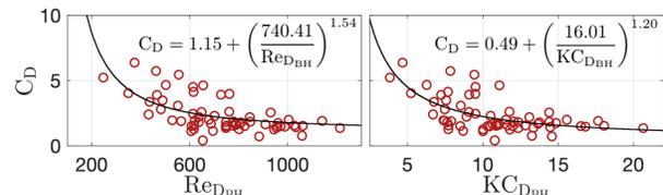
Figure 3 - Drag coefficients vs. Reynolds/KC numbers
