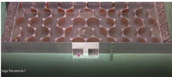
Figure 1 - Scale model example of an ARJ-R structure with long dissipative circuits made of circular cells with two frontal openings to the basin.
