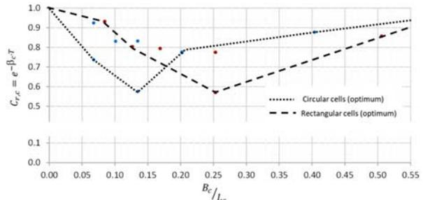
Figure 2 - Reflection coefficient of the ARJ-R structures related to the relative width of the dissipative chamber
