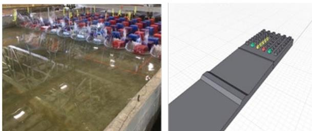
Figure 1 - A snapshot of wave impact on the structure (left) and computational domain for numerical simulation (right)
