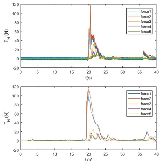
Figure 2 - Wave force on the structures: experimental results (top); numerical model results (bottom).
