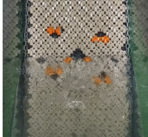
Figure 2 - Breakwater slope with clusters of extracted and broken XblocPlus units
