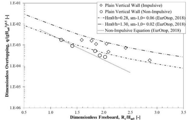
Figure 3 - Mean overtopping rates at plain vertical walls
