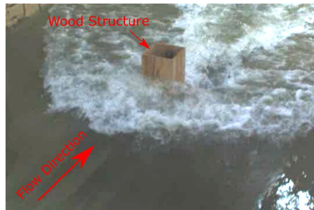
Figure 1 - Solitary wave impact on an idealized wooden structure.
