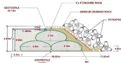
Figure 2: Design of protective measures.
