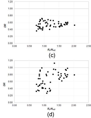
Figure 3. Variations of *DR* as a function of  $R_c/H_{m0}$  using the formulas of a) Postma (1989) b) Alikhani (2000) c) Zanuttigh and Van der Meer (2008) and d) Van der Meer and Sigurdarson (2016)
