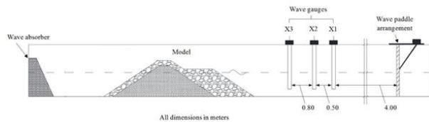
Figure 1 - Schematic cross section of the berm breakwater tested
