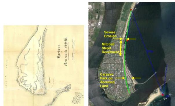
Figure 1 - Left: Entrance to Newcastle Harbour (circa 1850). Right: Present-day entrance with MEPBAY 1850 predicted shoreline superimposed indicating foreshore realignment and severe erosion and accretion.
