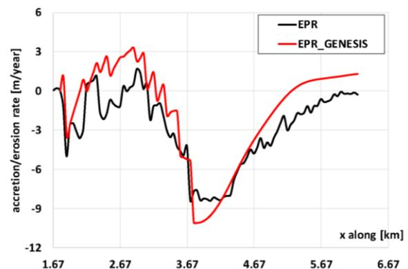
Figure 1. Comparison between measured and predicted EPR for the groins permeability  $P=0.2$  and for the  $K=0.2$ .
