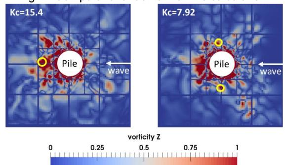
Fig. 2. Vorticity distribution in the  $z$  direction around the monopile (yellow circle: position of maximum scour depth in experiment)
