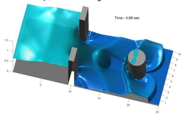
Figure 1 - Snapshot from a dambreak problem showing sharp shock fronts - computed by the GPGPU code.
