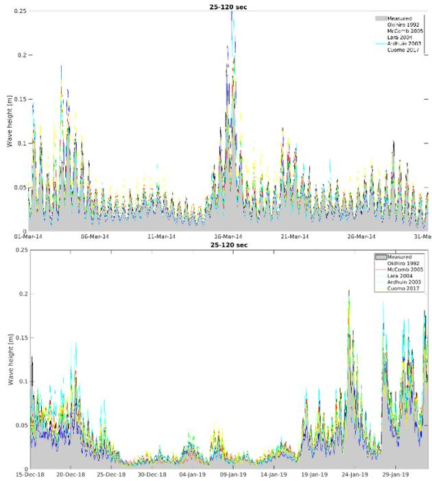
Figure 3 - Timeseries plots showing the measured and predicted IG significant wave heights for the five equations at Port Taranaki (upper) and Port Gijon (lower).
