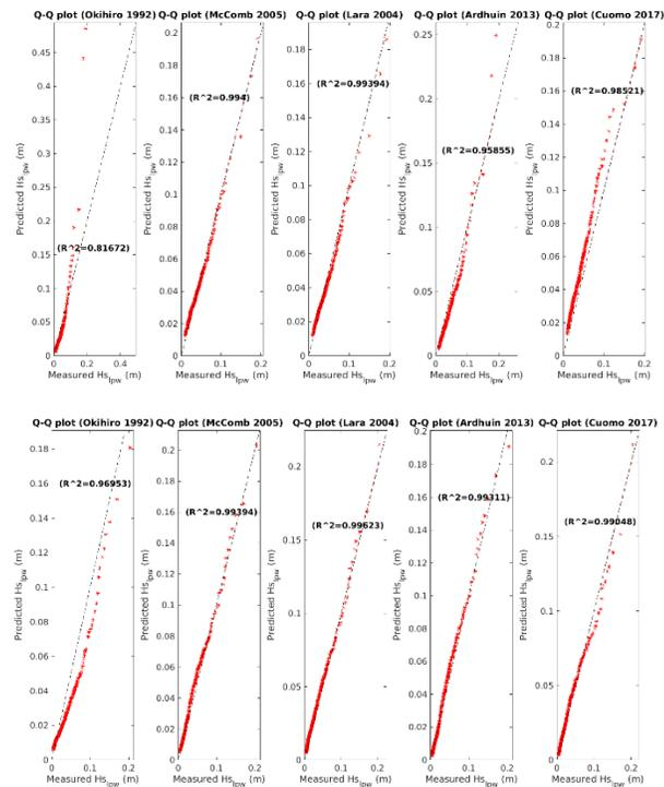
Figure 4 - Q-Q plots and associated linear regression coefficients for measured and predicted IG significant wave heights using the five equations at Port Taranaki (upper) and Port Gijon (lower).
