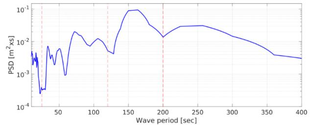
Figure 1 - Mean power spectra measured at Port Gijon, with annotation at 25, 120 and 200s period.
