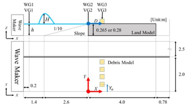
Figure 1 -Outline of experiment (h: water depth,  $Y_0$ : Initial distance in the Y direction from the reference point to the center of gravity of the drifting object)
