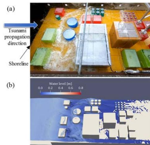
Figure 1 - (a) Image of the benchmark test, and (b) a snapshot of the water level predicted by the three-dimensional simulation.
