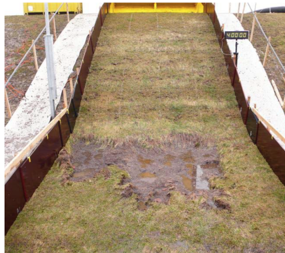
Figure 1: Grass cover erosion at the inner toe during wave overtopping tests on the Afsluitdijk (Bakker et al., 2009).
