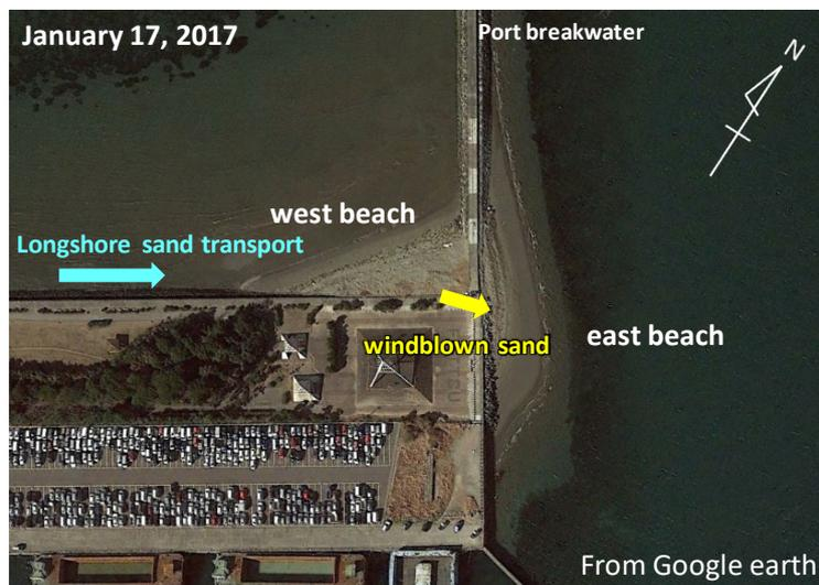
Figure 3. Satellite image of west and east beaches formed at corner between port breakwater and seawall.
