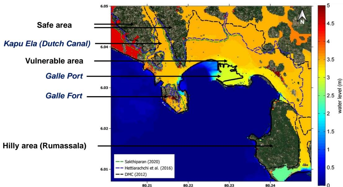
Figure 4: Simulated inundation together with inundation boundaries of previous studies (DMC 2012; Hettiarachchi et al. 2016 and Sakthiparan, 2020)
