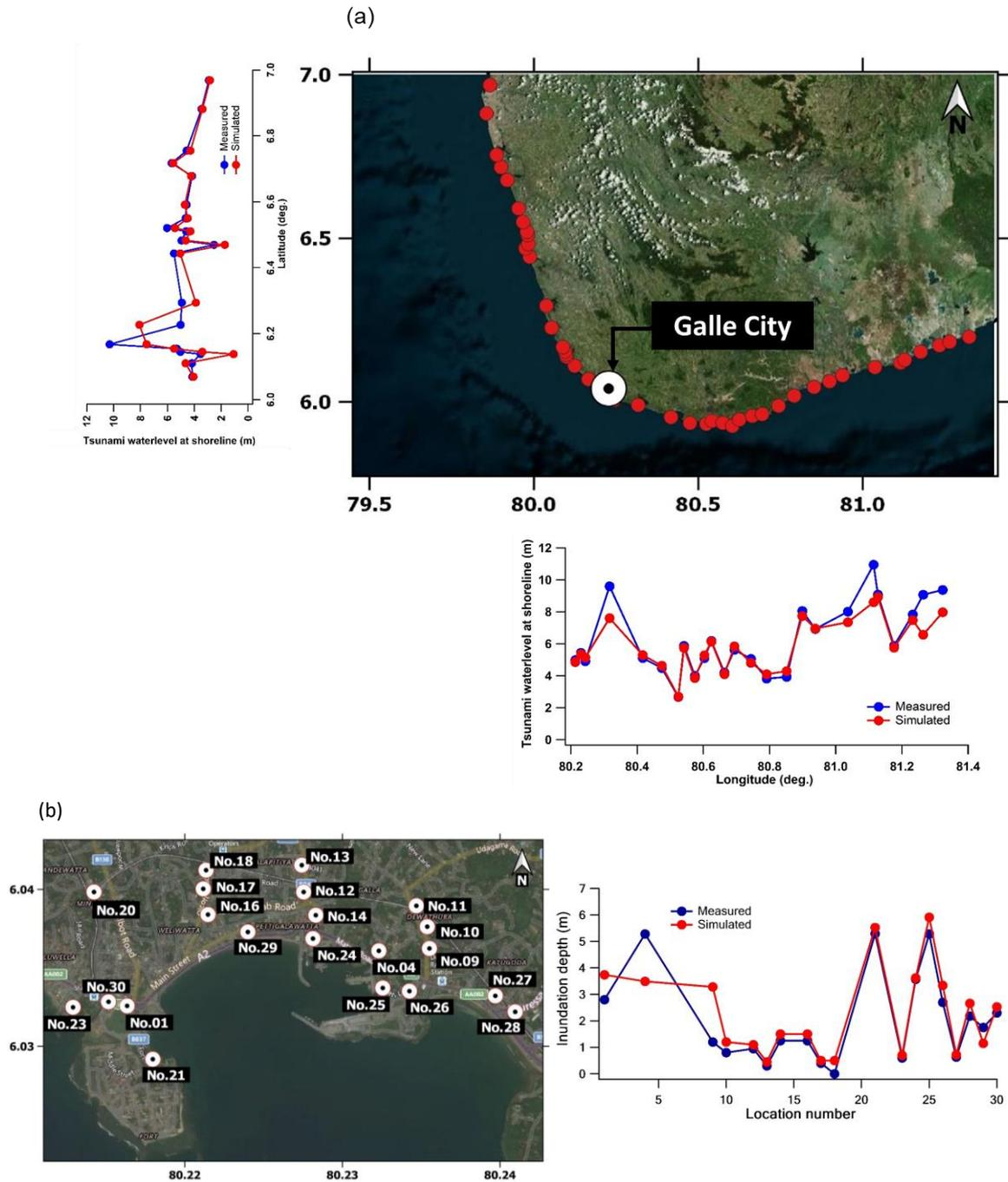
Figure 3: Model verification: (a) Comparison of simulated and measured water levels near coastline by Wijetunge (2006) (b) Comparison of field-measured inundation heights by Murata et al. (2016) with the simulation results.
