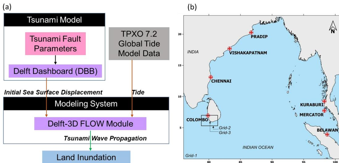
**Figure 2: (a) Modeling framework (b) Computational domain with tide gauges used to calibrate the model**
