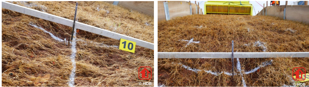
Figure 9. Test plot 4. Initial erosion hole after 6 hours with 50 l/s per m. The topsoil is largely eroded with the grass still maintained.
