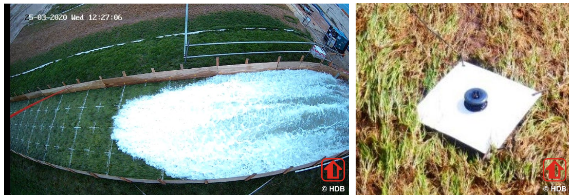
Figure 16. Left: an overtopping wave volume of 1500 l/m reaching the 12 m line 13 frames after reaching the 10 m line; front velocity 7.67 m/s. Right: Paddle wheels mounted on the grass slope, 3 cm above the slope.
