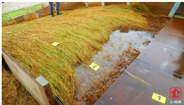
Figure 12. Test plot 6. Long grass (30-40 cm). Final situation after 200 l/s per m discharge at the crest.
