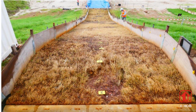
Figure 11. Test plot 5. The slope at the crest after 200 l/s per m, with the erosion area directly behind the crest.
