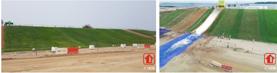
Figure 4. Overall view of Test plots 1-6, September 2019 (left). Overall view by drone of testing test plot 2. The tested Test plot 1 (brown grass) is on the left side and Test plots 3-5 on the right side.
