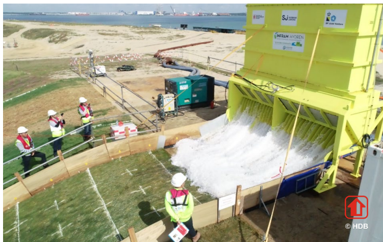
Figure 7. The wave overtopping simulator in action, taken by drone. The pipeline for water supply is shown in the background behind the simulator.
