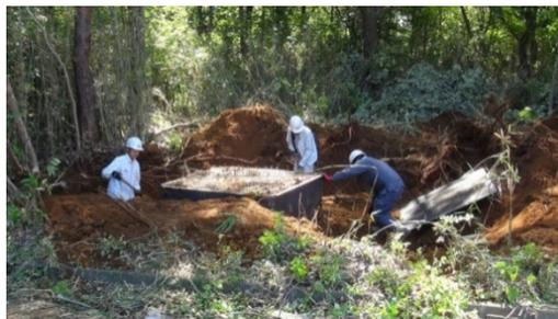
Figure 1. Collection of soil sample using the steel frame.
