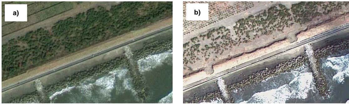
Figure 11. Erosion on sand bank (a) before the tsunami (16. Oct. 2009) and (b) after the 2011 Tohoku Tsunami (31. Mar. 2011).
