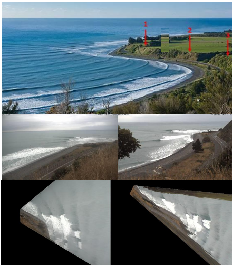
Figure 11. Location, field of view and rectified view of two remote camera systems installed at Mangamaunu
