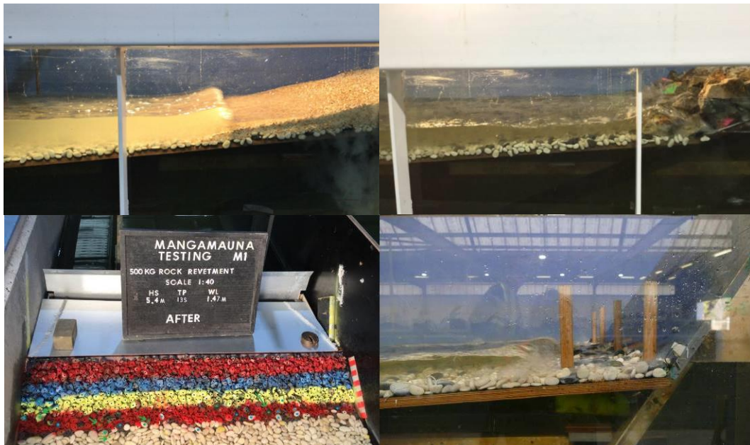
Figure 13. Physical modelling testing of the existing boulder beach (top left), a 2T rock armour revetment (top right) with optimization of the rock revetment (lower left) and testing of a piled structure (lower right)
