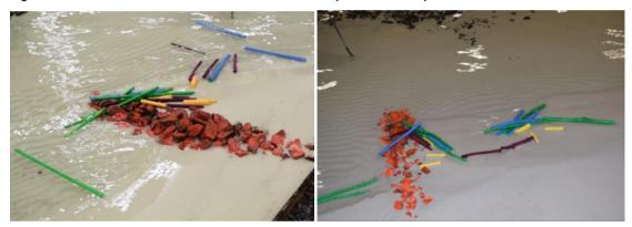
Figure 2. Model woody debris: dowels (left) and tree branches (right).
