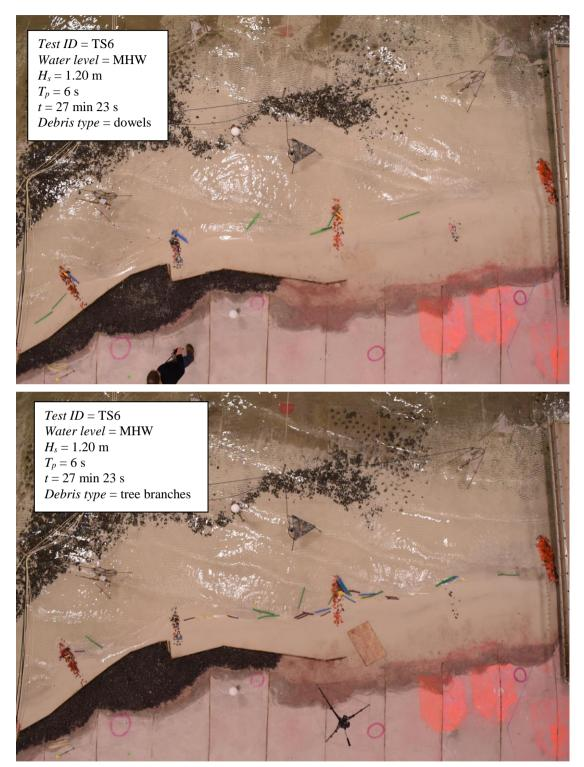
Figure 6. Snapshots (at t = 27 min 23 s) of experiment TS6 with dowels (top) and branches (bottom), illustrating the effects of debris morphology on mobility.
