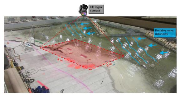
Figure 1. Overview of the 1:30 scale coastal model and experimental setup.
