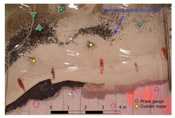
Figure 3. Locations of wave probes and current meters.
