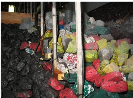
Figure 7: Detail of pressure sensors between core and filter layer
