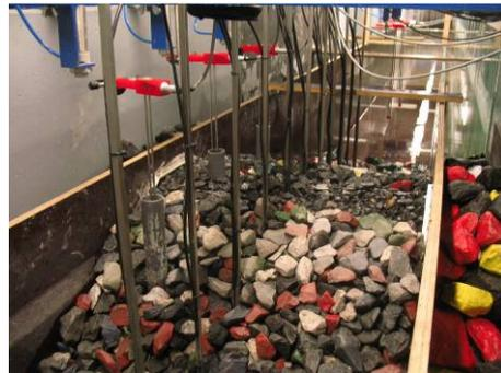
Figure 6 : Wave gauges in perforated tubes (stage 2)
