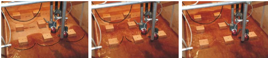
Figure 9. Three snapshots of the run-up process in chronological order from left to right, obstacles consist of wooden blocks with edge length of 10 cm at a distance of 15 cm
