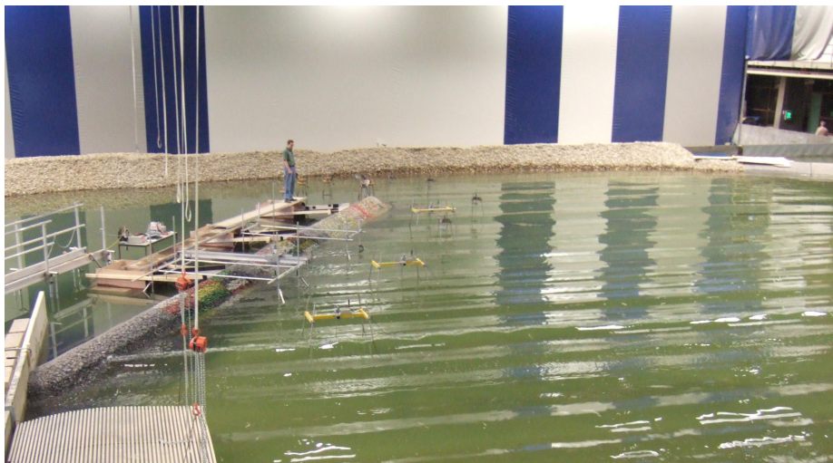
Figure 1. Breakwater in wave basin
