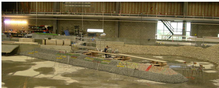
Figure 2. Overview of breakwater model in wave basin.
