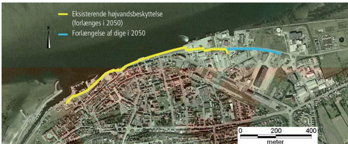
Figure 8. Strengthening of flood protection by raising the sea wall 0.4 m and extending it towards east
