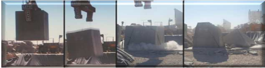
Figure 9. Anvil Drop (AD) of conventional cubic block CAU ( h[m]=2.0 , n=1 ).
