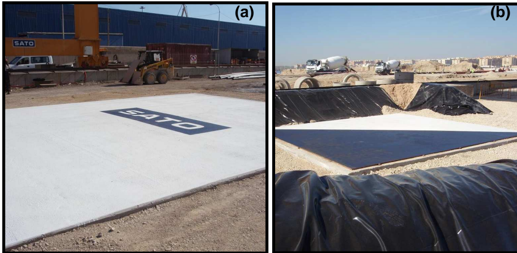
Figure 6. Reinforced-concrete platforms: (a) Overturning tests and (b) Free fall tests.
