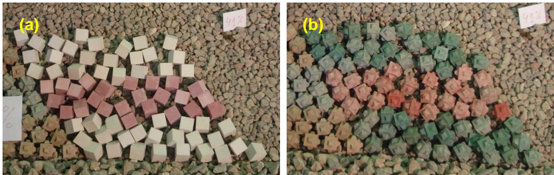
Figure 12. Realistic 3D CAU placement, on H/V=3/2 slope, using a small-scale crawler crane with CBPS positioning grids: (a) cubes, and (b) Cubipods.
