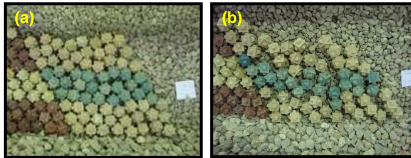
Figure 10. Cubipod armors with CBPS: (a) minimum porosity p\%=37\% , and (b) maximum porosity p\%=51\% .
