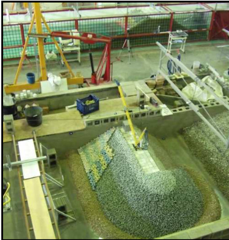
Figure 15. General view of ongoing 3D placement and 2D hydraulic stability tests of H/V=2.0 slope models.
