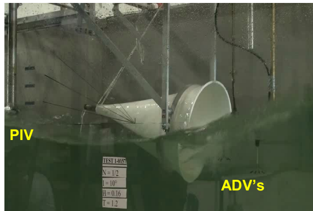
Figure 9. Blow-Jet during tests.
