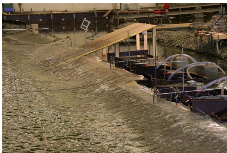
Figure 3. Overall view of the Flowdike model with two crest heights and the run-up board.
