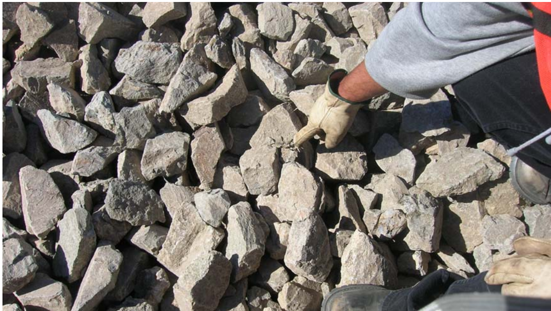
Figure 7 Visual Appearance – 100mm Single Size Granular Bedding Material (Post Test)
