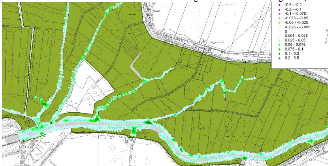
Figure 15: Delta of bed evolution and its sensitivity due to higher SPM-influx at the tidal boundary +150 mg/l in [m/4 month]
