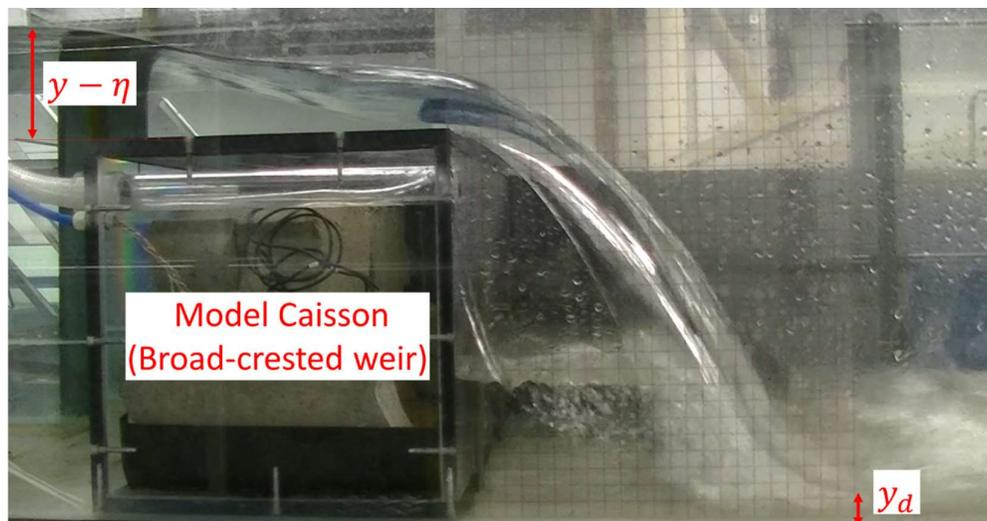
Figure 8b. Supercritical flow downstream when the downstream water depth is less than the critical depth
