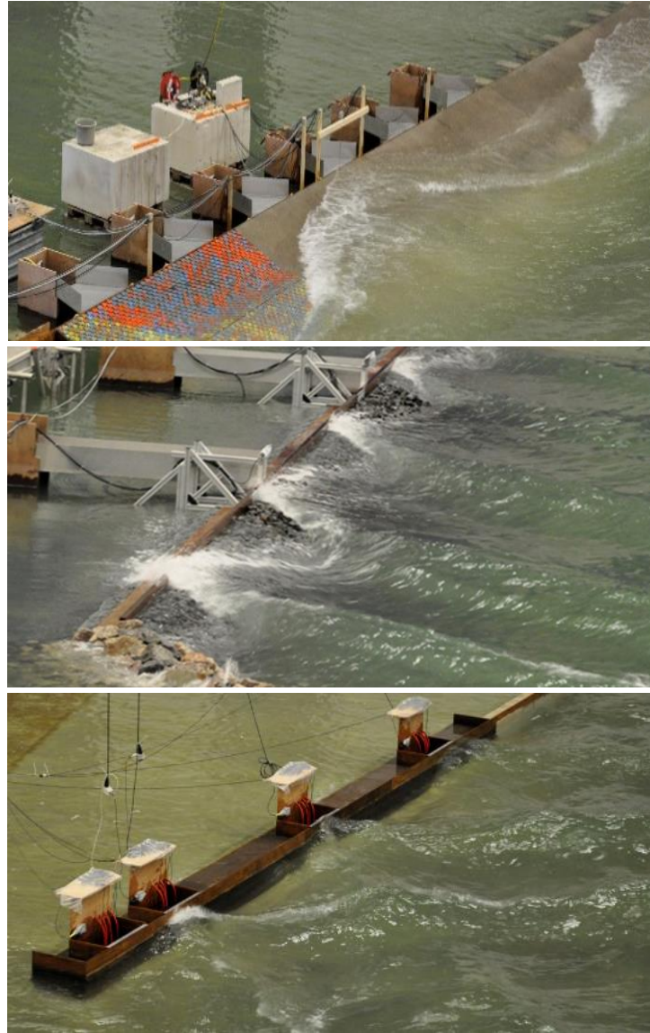
Figure 1. Pictures of model tests in a wave basin with oblique wave attack on a sloping dike (upper panel), rubble mound breakwater (mid panel), and a vertical caisson breakwater (lower panel); source: Van Gent and Van der Werf (2019) and Van Gent (2020, 2021).
