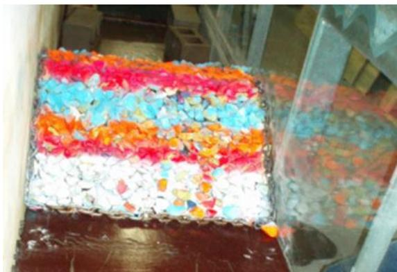
Figure 3b Model T1 Section A2 after test 10 – Hs = 4.56m, Tp = 14.07s, damage 9.5%
