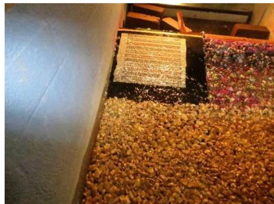
Figure 3c comparing wave runup on permeable (rhs rock) and impermeable structure (lhs wood)
