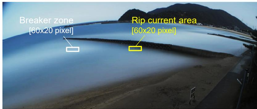
Figure 15. Pixel value comparison areas set for wave breaking zone and rip current area in the averaged image of Cam 3.
