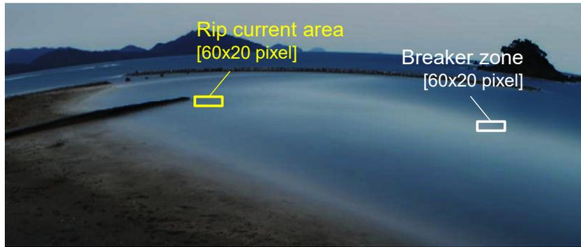
Figure 18. Pixel value comparison areas set for wave breaking zone and rip current area in the averaged image of Cam 4.
