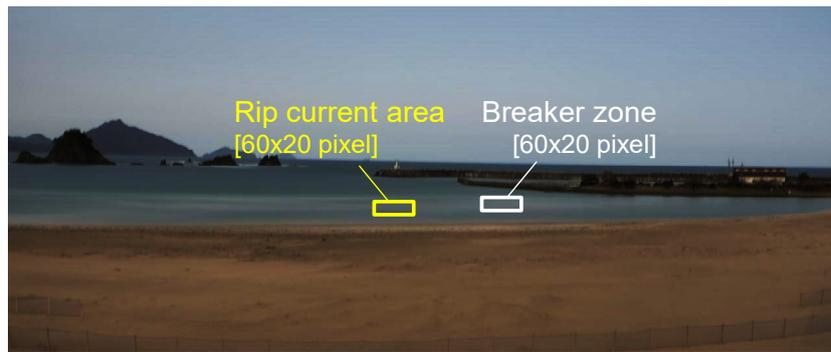
Figure 13. Pixel value comparison areas set for wave breaking zone and rip current area in the averaged image of Cam 1.
