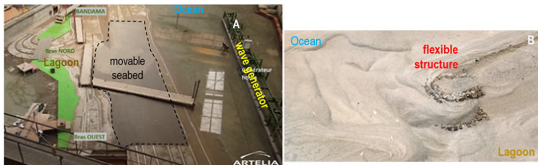
Figure 11. View of the physical model (A) - View of the bottom of the future fishway and the bank retaining structure after 3 annual cycles.
