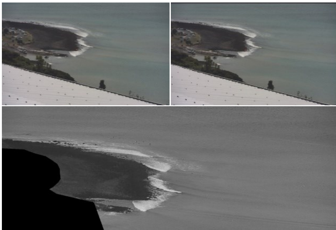
Figure 2. Original FoV image from 1300 hrs on the 30 th November 2017 (top left), registered image showing slight right to left and up down shift in camera (top right), and grey scale version of the registered image that is cropped and masked (bottom). Note the orange (top row) GCP flag left of centre.
