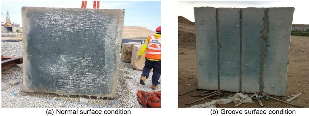
Figure 9. Concrete surface roughness conditions
