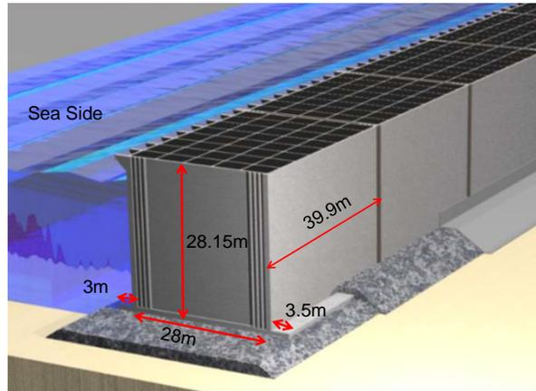
Figure 5. Typical caisson dimensions
