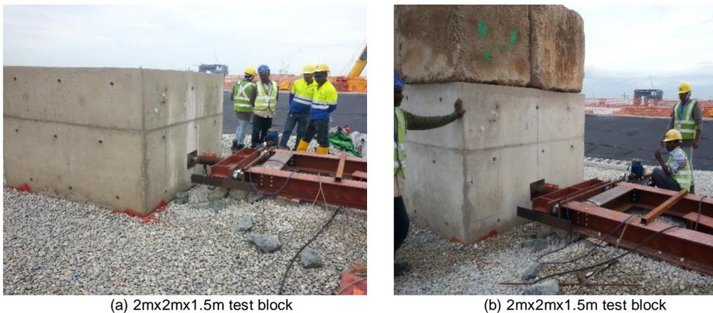
Figure 10. Vertical load conditions for test blocks
