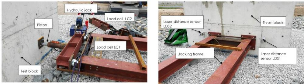
(a) Test blocks and load cells
