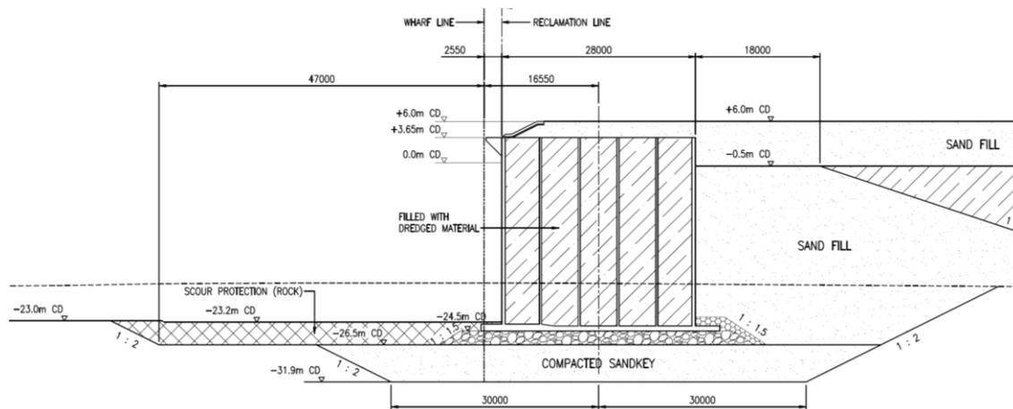
Figure 4. Typical cross section for caisson system with compacted sandkey
