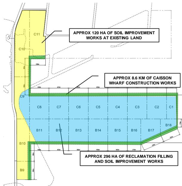
Figure 2. Layout Plan and General Scope of Works for Tuas Port Phase 1
