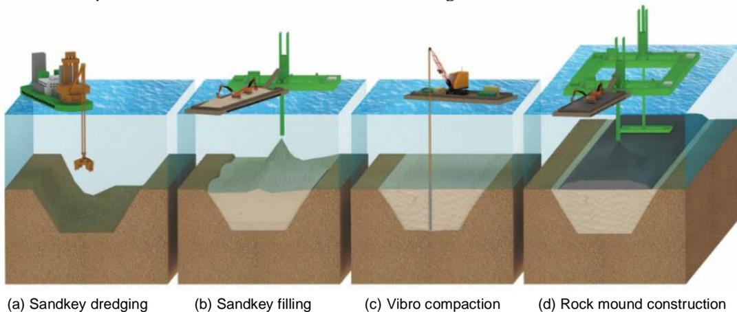
Figure 6. Typical construction sequence of caisson foundation
