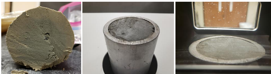
Figure 15. Testing of a sample taken from the boulder clay layer at Den Oever.
