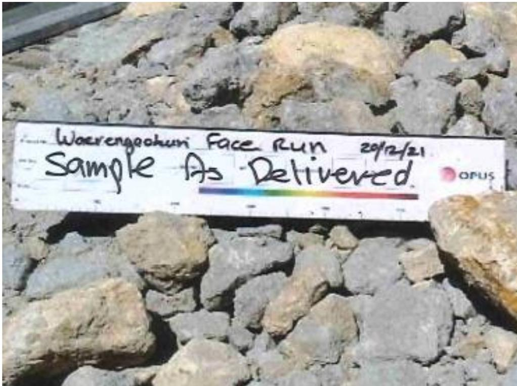
Figure 2. Quarry run sample used in hydrometer analysis
