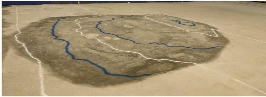
**Figure 15. Completed mound with blue and white alternating contour lines indicating elevations corresponding to -5 (small blue crest line, right side of image), -6, -7, -8, -9, and -10 (far left white line) m AHD.**
