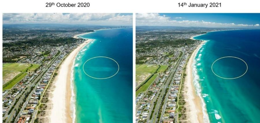
**Figure 12. Mound is visible approximately eight weeks after placement (left) and subsequently engulfed by the storm bar (right) following the December and January storms. Yellow circles assist in showing the approximate mound location for comparison of the two images.**
