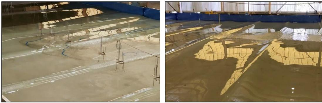
Figure 17. The top photos depict the wavefield in the baseline, no-mound conditions during TS1. With no mound, the waves can be seen to be breaking relatively uniformly in the longshore. The bottom photos show the wavefield with the first mound in place. The presence of the mound resulted in more variability in the breakpoints with the larger waves breaking over the mound (lower left image) and smaller waves breaking in the lee of the mound, demonstrating the focussing effect.
