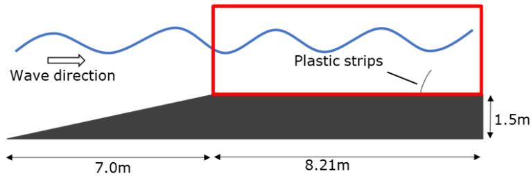
Figure 2. Physical modelling setup of Paul et al. (2016) with numerical domain highlighted in red.
