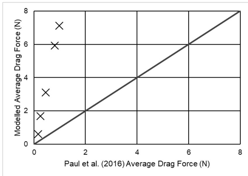
Figure 6. Modelled vs. measured average drag force.
