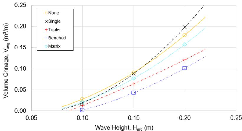
Figure 13. Comparison of volume change,  $V_{avg}$ , for each LWD configuration under the base set of three wave conditions. Dashed lines are fitted second-order polynomials.
