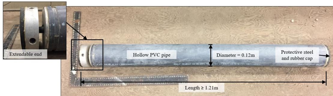
**Figure 2.** Model log, manufactured with hollow PVC piping, steel caps, and rubber ends. One end extends to provide lateral pressure and fix the log in place.
