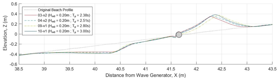
Figure 8. Influence of wave period on the equilibrium beach profile. Tests with varying wave period and constant wave height for a Single LWD structure (03-v2, 04-v2, 09-v1, and 10-v1).
