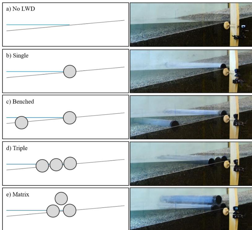
**Figure 3.** Test configurations. Conceptual sketches (left) and photographs of the experimental set-up (right).
