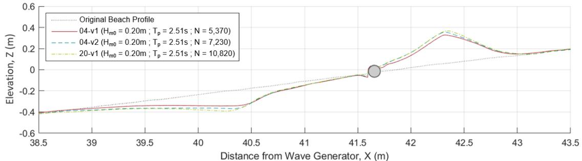
**Figure 6. Influence of simulation duration on the equilibrium beach profile. Tests with varying duration (e.g. number of waves) and constant incident wave conditions for a Single LWD structure (04-v1, 04-v2, 20-v1).**
