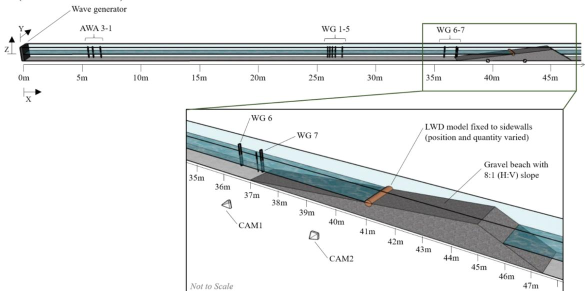
**Figure 1. Schematic of experimental set-up (not to scale).**
