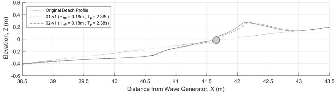
**Figure 5. Comparison of the equilibrium beach profile for repeated tests for a Single LWD structure (01-v1 and 02-v1).**
