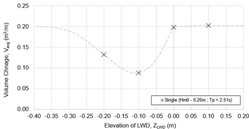
**Figure 15.** Influence of LWD elevation (relative to the water level at  $z = 0.0$  m) on volume change,  $V_{avg}$ , for the base case scenario (single LWD with target wave characteristics:  $H_s = 0.2$  m and  $T_p = 2.51$  s). The gray dashed line is a hand-fitted theoretical relationship between LWD elevation and volume change.
