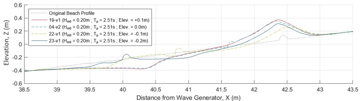
**Figure 11. Influence of LWD elevation relative to the still water level on the equilibrium beach profile for a Single LWD structure (19-v1, 04-v2, 22-v1, and 23-v1).**
