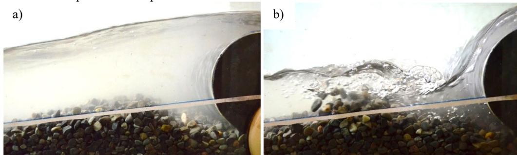
Figure 14. Close-up image of scour formation seaward of a LWD structure, during (a) wave run-up and (b) run-down
