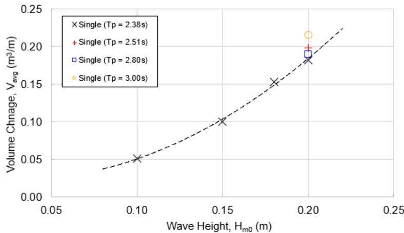
Figure 9. Influence of wave height,  $H_{m0}$ , and wave period,  $T_p$ , on volume change,  $V_{avg}$ , for a Single LWD structure. Dashed line is a fitted second-order polynomial for a constant wave period of  $T_p = 2.38s$ .
