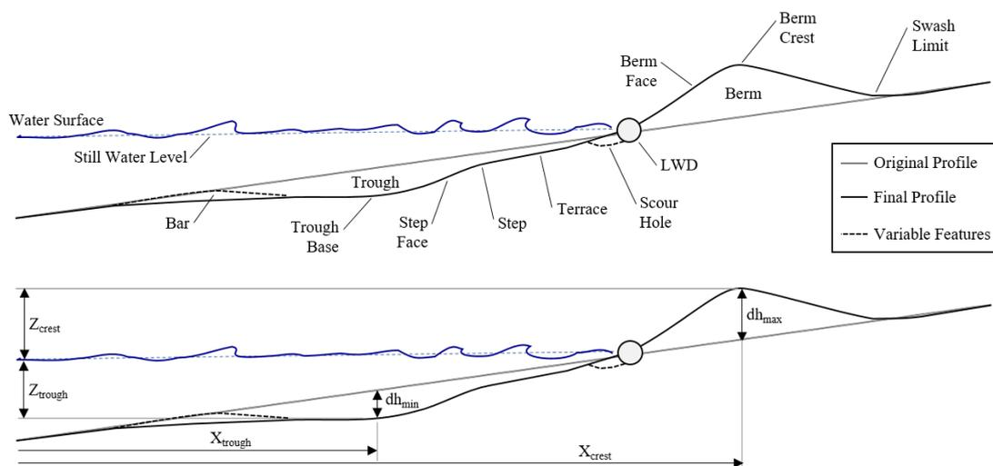
Figure 4. Beach profile characteristics (top) and variables (bottom) (adapted from USACE, 2002).
