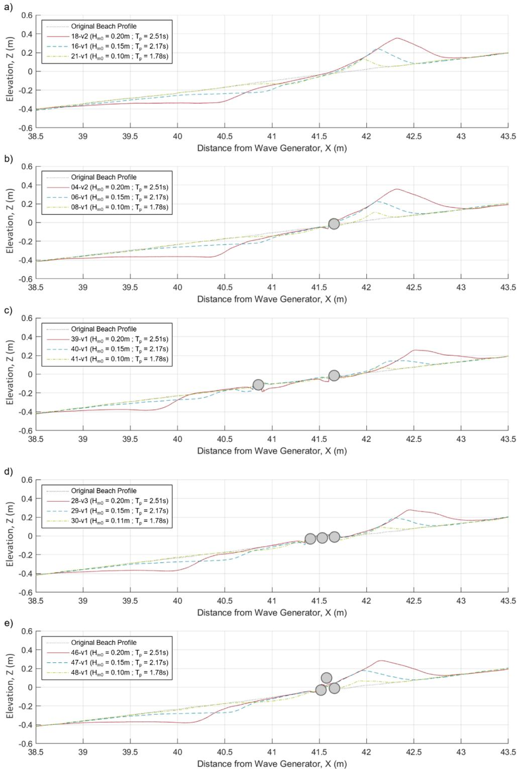
Figure 12. Influence of the LWD design configurations on the equilibrium beach profile under the three base wave conditions, for: (a) None, (b) Single, (c) Benched, (d) Triple, and (e) Matrix-style LWD structures.
