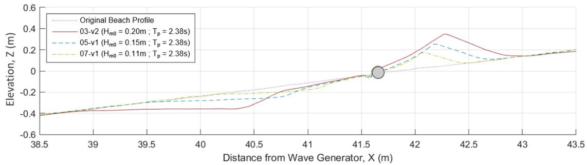
Figure 7. Influence of wave height on the equilibrium beach profile. Tests with varying wave height and constant wave period for a Single LWD structure (03-v2, 05-v1, 20-v1).
