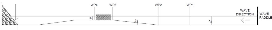
Figure 1. Schematic diagram of experimental setup.
