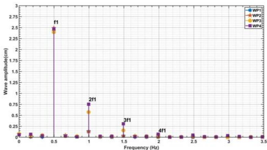
Figure 5. Frequency analysis for the waves at corresponding wave gauges.
