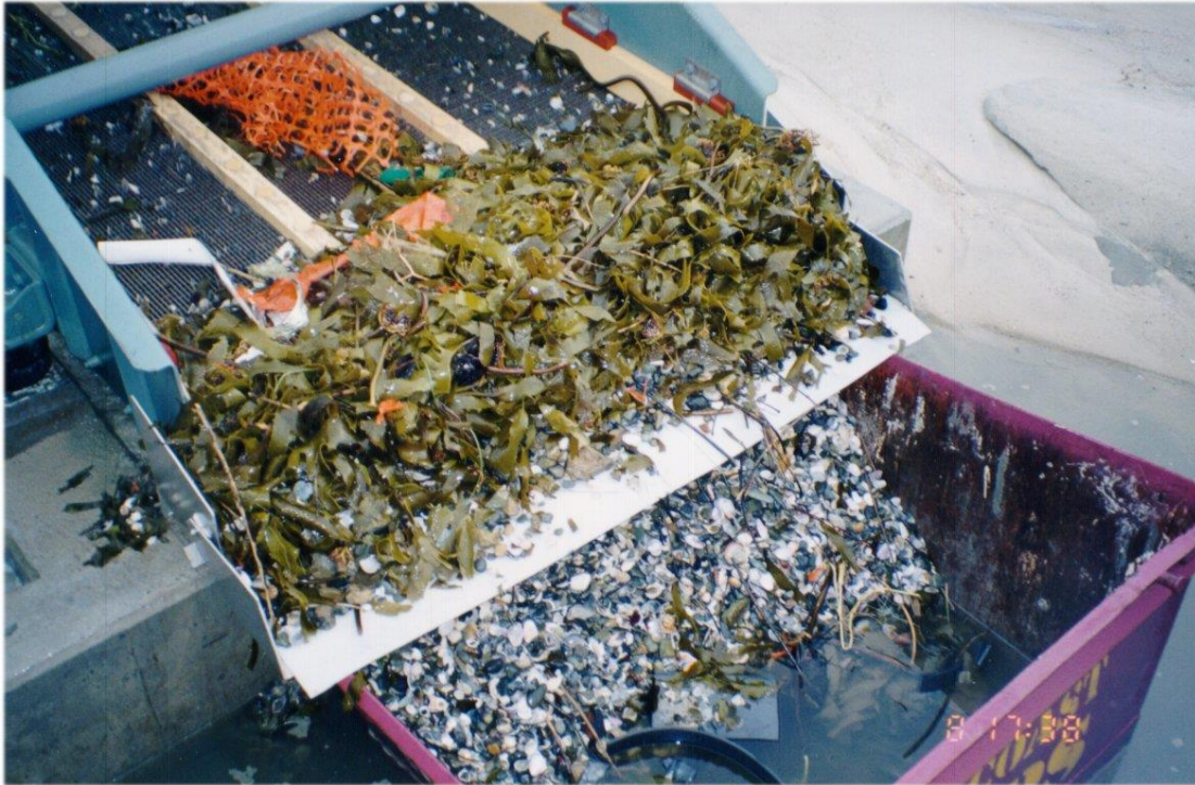
Figure 10. TRESBP in Australia. Vibrating harrowing screen, stones and pebbles extracted from the mixture, wood fragments next to the extraction cones and large trunks in the sand trench.
