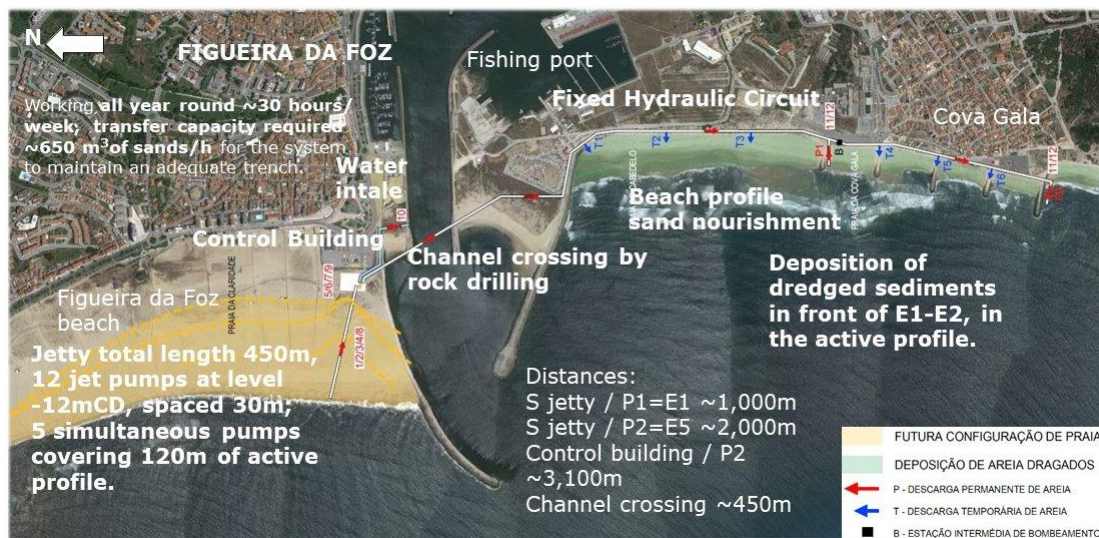
Figure 4. Figueira da Foz. Fixed ASBP solution: sand collection, control building, hydraulic circuit crossing the channel and fixed discharge pipeline. Source: Carvalho et al. (2021).
