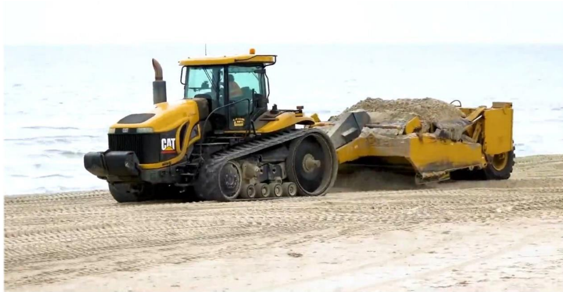
Figure 6. ASBP mixed system – Adelaide Beaches, Australia – scraper recovering sand.
