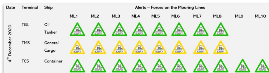
Figure 6. Dashboard of the alerts for the forces on the ships' mooring lines.
