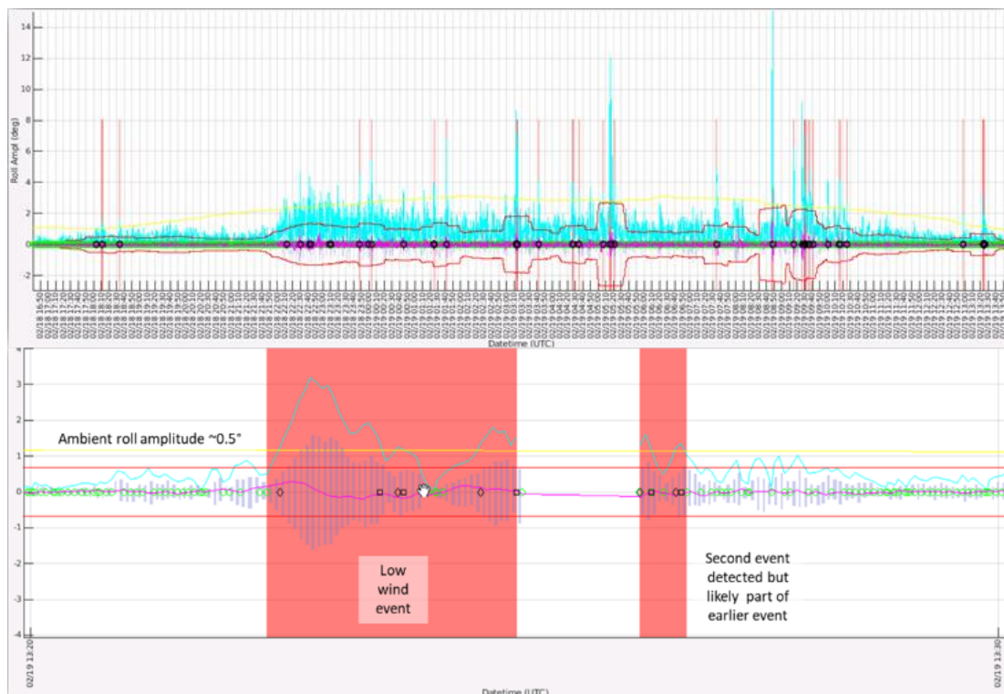
Figure 3. Dynamic threshold event detection algorithm to distinguish between boat motion 'events' and motions in the background sea state
