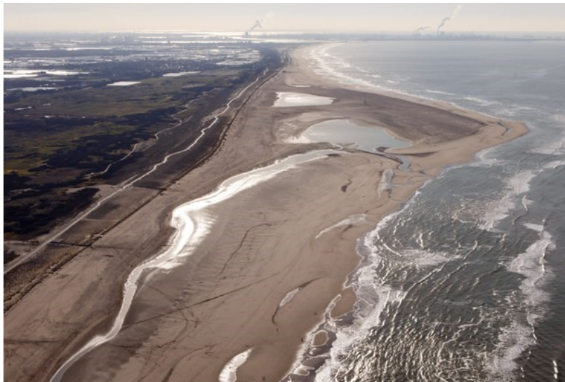
Figure 1. Example of Type 1 Coastal NBS – Expansive. The Sand Motor in the Netherlands. This project is a mega scale beach renourishment project. The project placed 21.5 million m 3 of sand in a hook-shaped peninsula of 128 ha, including a dune lake and a lagoon. Following construction in 2011, the sand has indeed spread along the coast, with coastal accretion both to the south and the north. Photo credit: Rijkswaterstaat/Jurriaan Brobbel.
