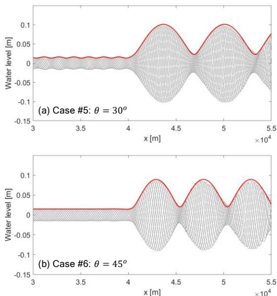
Figure 6 - Comparisons between the simulated water levels and the theory for obliquely incident wave groups over a plane beach. Red: Envelope height of the wave surface based on the theory of Liu (1989). Black: Simulated wave surface elevations.
