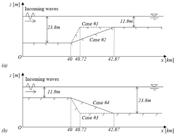
Figure 3 - Bathymetry of the plane slope beaches.
