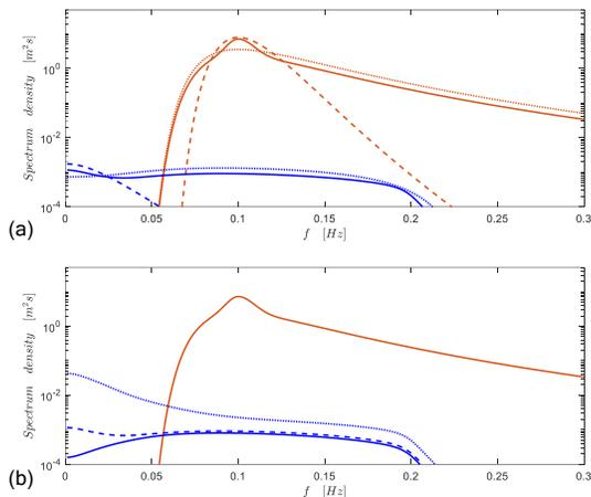
Figure 2 - Spectra of free/input waves (red line) and the bound IG waves (blue lines). In (a): Dot - PM spectrum; Solid - JONSWAP with  $\gamma = 3$ ; Dash - Wallops with  $m = 20$ . In (b): Solid -  $h=100\text{m}$ ; Dash -  $h=50\text{m}$ ; Dot -  $h=20\text{m}$ .
