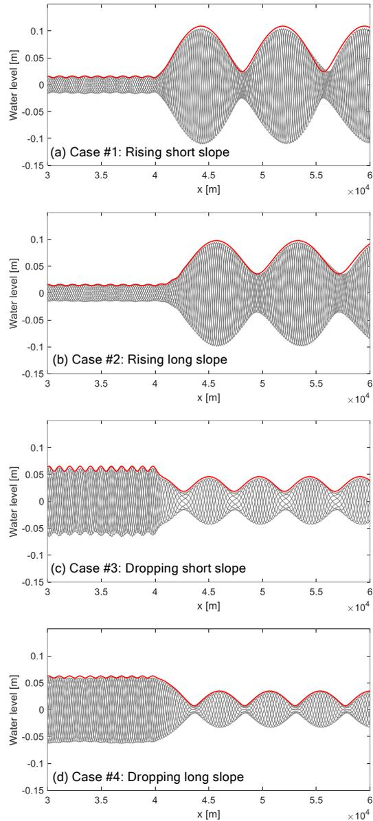
Figure 4 - Comparisons between the simulated long waves and the theory for plane slopes. Red: Envelope height of the wave surface based on the theory of Liu (1989). Black: Simulated wave surface elevations.
