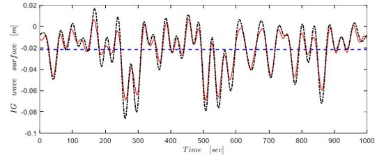
Figure 1 - Comparisons of IG wave surface. Red: Present theory; Black: Second-order potential flow theory; Blue dash line: Radiation stresses induced mean set-down.
