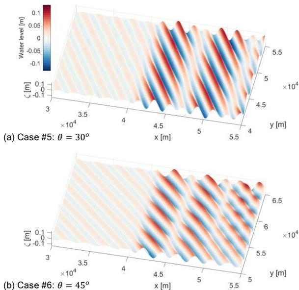
Figure 5 - Simulated long wave surfaces for obliquely incident short wave groups.
